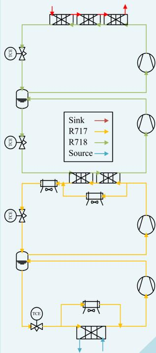
Intermediate pressures and temperatures are optimised for highest COP.
